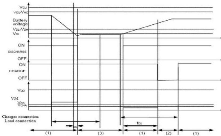
Notes: (1) Normal condition (2) Overcharge voltage condition (3) Overdischarge voltage condition
